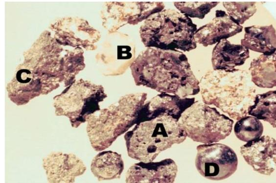
(b) Fragments of the main types of lunar rocks: basalt (A), anorthosite (B), and breccia (C), glass spherules (D).
