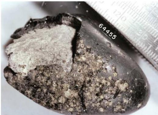
(a) Glass-coated basalt melt sample no. 64455
