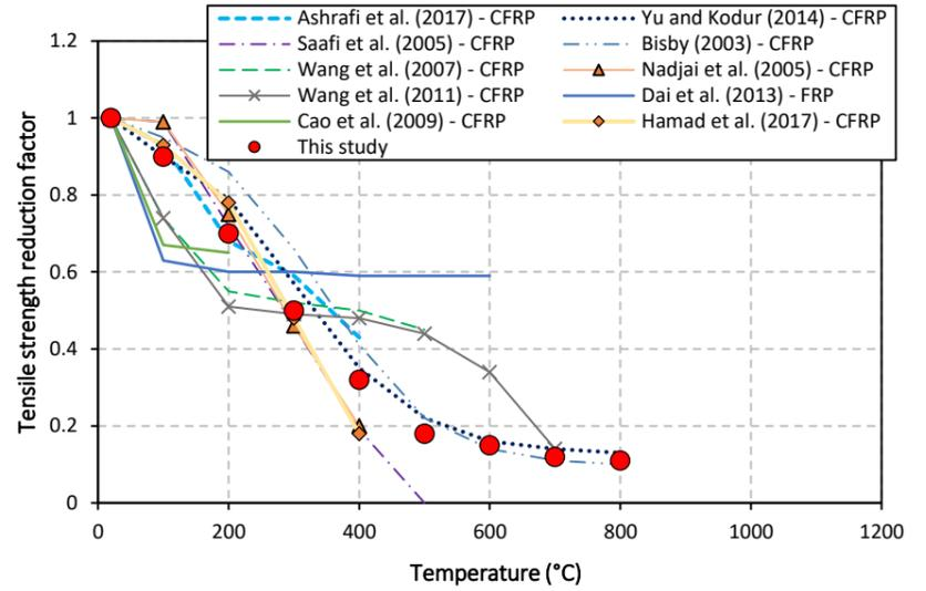
(h) Fiber-reinforced polymers (CFRP)
