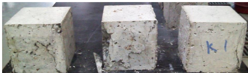
(d) Specimens contaminated with 1.0% kerosene at 14 days
