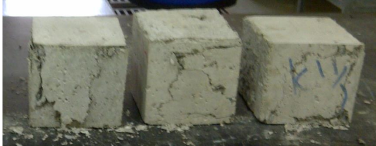
(a) Specimens contaminated with 1.5% kerosene at 28 days Fig.5. Failure mode of the tested specimens
