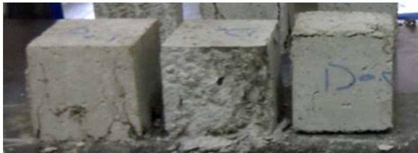
(b) Specimens contaminated with 0.5% diesel at 7 days
