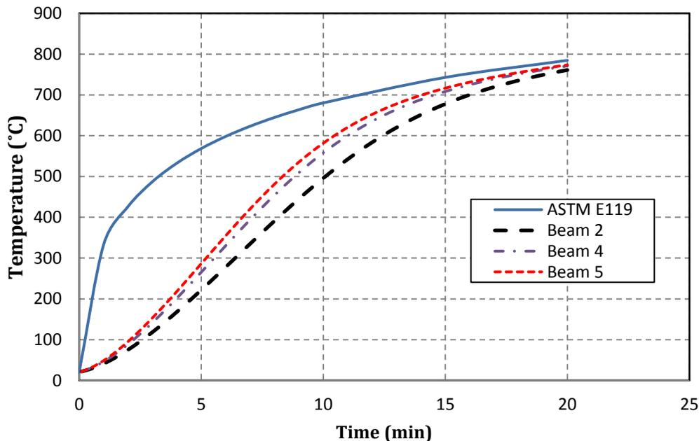
Fig. 10. Variation of temperature in web of Beams 2, 4 and 5 with fire exposure time
