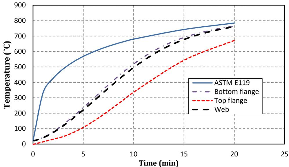
Fig. 7. Temperature in steel beams 1, 2 and 3 as a function of fire exposure time
