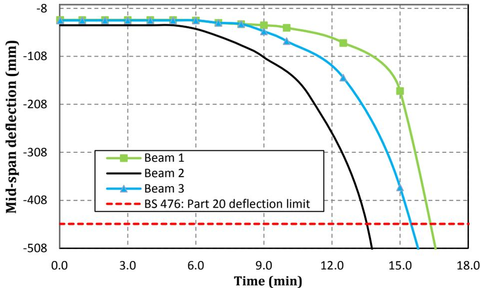
Fig. 9. Variation of mid-span deflection with fire exposure time in “Beam 1”, “Beam 2” and “Beam 3”
