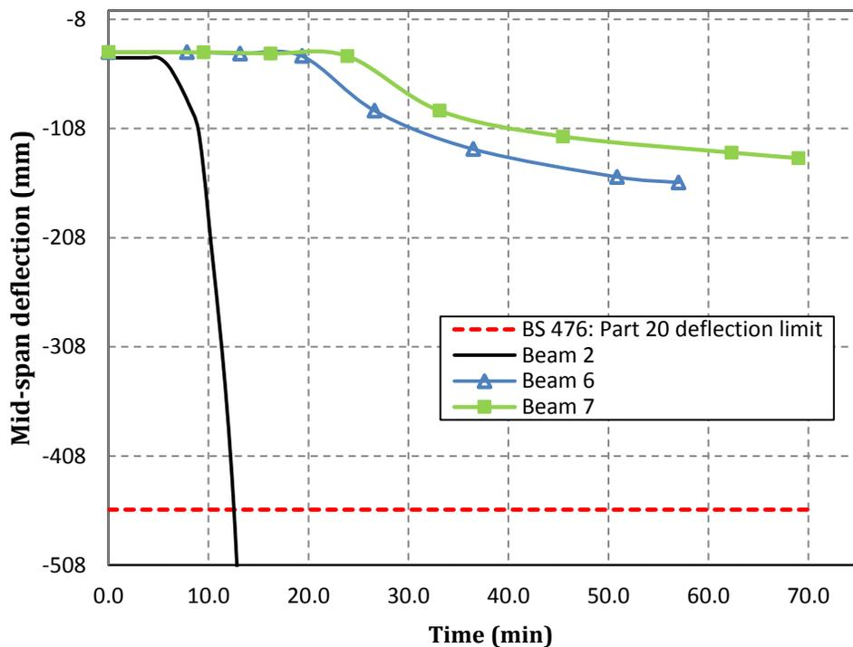
Fig. 16. Comparison of mid-span deflection in Beams 2, 6 and 7
