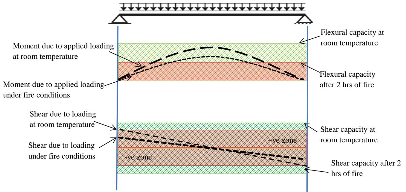
(a) Beam with uniformly distributed loading at ambient and fire conditions
