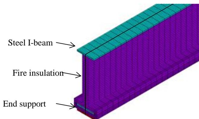
Fig. 13. Detailed view of fire insulated steel “Beam 6”
