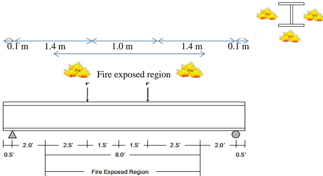
Fig. 3. Tested beam used in validating the developed finite element model
