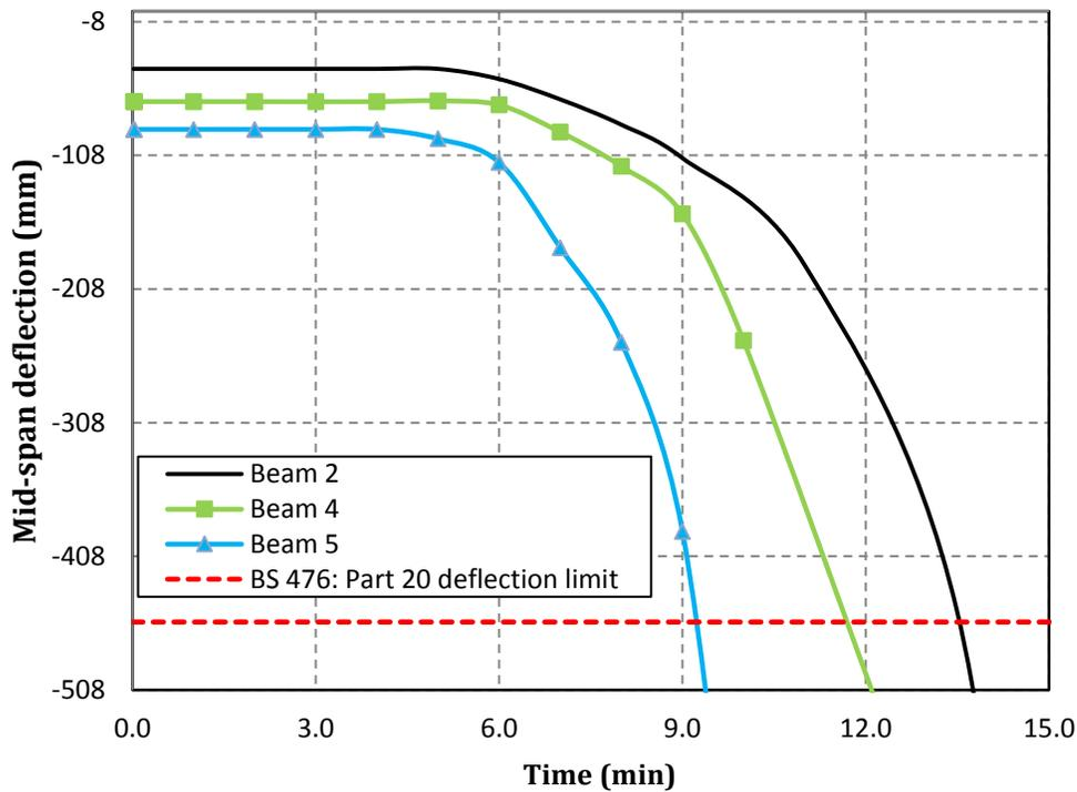
Fig. 12. Comparison of mid-span deflections in Beams 2, 4 and 5 with different web slendernesses
