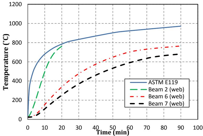
Fig. 14. Predicted temperature propagation of Beams 2, 6 and 7
