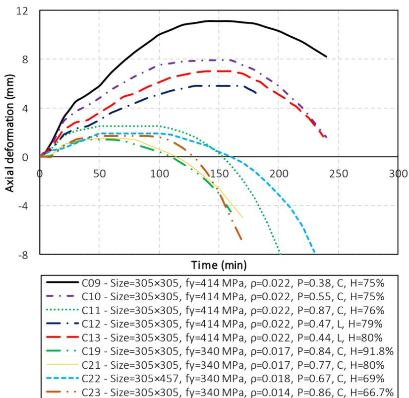
(c) Measured response of carbonate and lightweight RC columns
