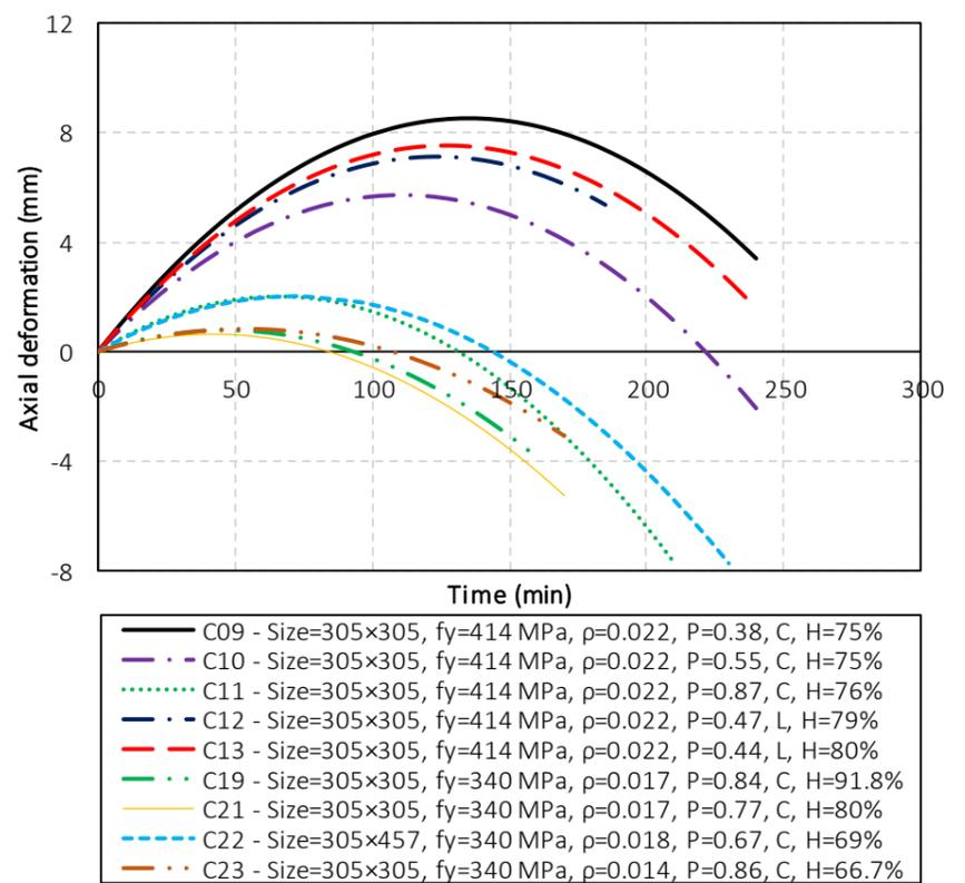
(d) Predicted response of carbonate and lightweight RC columns
