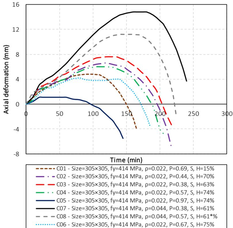
(a) Measured response of silicate RC columns
